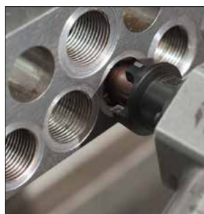
Safely re-machine gasket surfaces in seconds.
