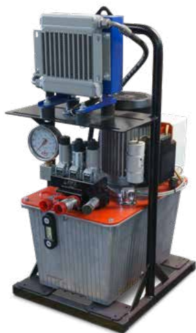
ELECTRIC 230 V WITH OIL COOLER
